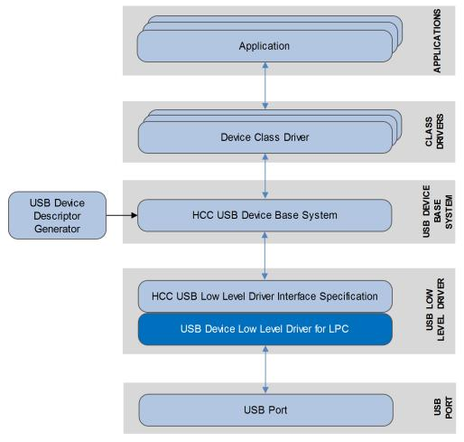
The low level driver is always started automatically by the USB device stack. The driver is linked to the stack at compile time because each low level driver uses the same function names. This also means that only one driver can run in a system.
