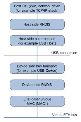
The USB device port creates a virtual Ethernet port on the embedded device. This connects to a physical Ethernet port and thus to a network. If the embedded device wants to be a device on that network then we provide a virtual network on the embedded device - so that the network driver logically talks to another virtual Ethernet port inside the device - and a network stack can then be built on that interface.
