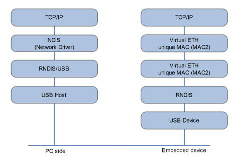
This class driver is effectively a library. It provides a set of function calls that an application can use to send and receive data through the serial port. The **usbd\_rndis\_init()** function registers the class driver with the Embedded USB Device (EUSBD) base system and this call sets up callbacks for the base system to use.
