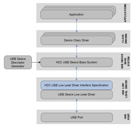
A driver must be written specifically for a particular USB device controller. Each implementation is designed to work with the USB device core (the base system).
