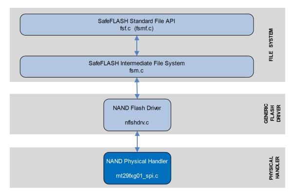
The main SafeFLASH package provides the file API and intermediate file system. This is described in the HCC SafeFLASH File System User Guide. This design is highly portable and gives excellent performance. The basic device architecture includes a high level driver for each general media type that shares some common properties. This driver handles issues of FAT maintenance, wear leveling, and so on.
