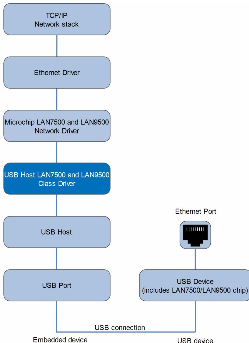
The host implementation allows the host system to transfer Ethernet packets to/from a remote Ethernet port at the other end of the USB connection. It connects to a USB device that has an Ethernet port on it that connects to a real or virtual network.
